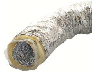
sotherm Light / Sonotherm Light are flexible thermally (Isotherm) and thermally and acoustically (Sonotherm) insulated ducts used as connection elements for transporting air in ventilation and air-conditioning systems. They perfectly suppress noise, eliminate vibrations, and reduce the need to use fittings.
